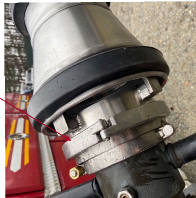
Attach nozzle flange to aerator flange. Capture both with hinged mounting collar. Snug tight thumb screw. If permanent, use blue lock tight on thumb screw threads.
