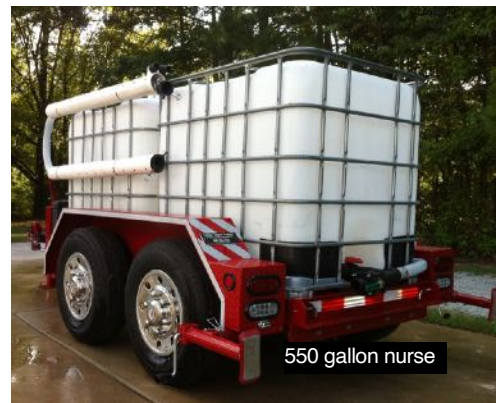
275, 330, 550, 660 or 990 gallon FoamChariot nurse. Transfer pump only, no firefighting station,
