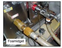
tube. When you need class B foam, put the eductor on any discharge and connect the pick-up tube to the foam tank line. When the tank is empty, disconnect the tube from the tank outlet and use foam pails or a drum to keep the system going. Flush it by sucking up five gallons of fresh water. If you are using TFT's new self-flushing foam eductor, simply push the flush button, which cleans interior works of the eductor and pickup tube. There is no need to disassemble or bucket flush this one.
