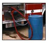
pumper in your fleet into a crash truck. SSE's have one moving part. (no pumps or flow meters.) These devices use the fire pump energy you already bought to drive them. The difference between one of these and a discharge side
