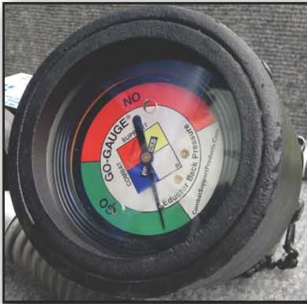
Hardened gauge enclosure with 3/16" vented Lexan cover
