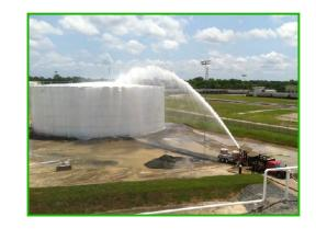
Type II applications include those that one would use on foam destructive fuels such as polar solvents or some acids. Using bank-in (back-splash) off the side of wreckage or roll-on using nozzle velocity to push foam onto a fuel spill or fire somewhat gently.
