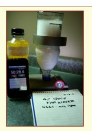
Test your foam and system: Take concentrate sample from your engine's foam tank and the water from its booster tank. Do the 3% bottle shake and record the time.
