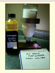
Test your foam and system: Take concentrate sample from your engine's foam tank and the water from its booster tank. Do the 3% bottle shake and record the time.
